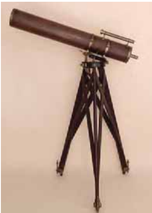
289. ADAMS REFLECTING TELESCOPE, circa late 1800's , mahogany telescope with brass fittings mounted upon a fixed-leg mahogany tripod with adjustable universal telescope mount and leveling legs, made in London, England. Tripod Height 51 ½ in. Scope Length 49 ½ in. Scope Diameter 6 ½ in.
